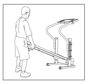
2. Move your right hand to the position shown and hold the treadmill firmly. Using your left hand, pull the latch knob to the left and hold it. Raise the treadmill until the pin on the latch knob is aligned with the latch hole in the frame. Slowly release the latch knob. **Make sure that the pin is inserted into the latch hole in the frame.**
